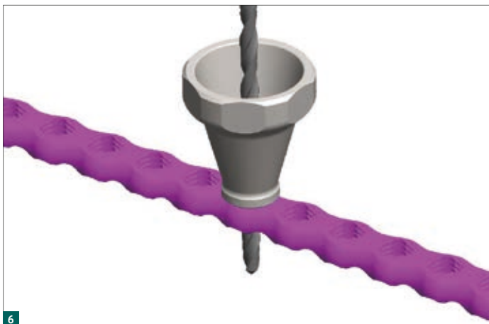
Fig. 6: The drill guide funnel is screwed vertically into the plate hole thread. With the twist drill, the inclination of the locking screws can be determined (up to \pm 15^\circ longitudinal and transverse pivoting).
