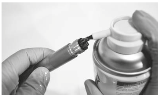
Injecting maintenance oil into the spray channel (maintenance oil item no. 174010 and spray channel adapter item no. 17401150)
