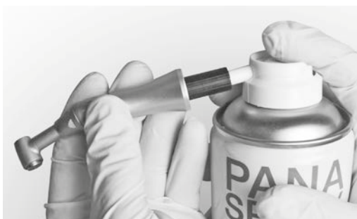
Injecting care oil into handpieces with a planar receiving shaft (care oil item no. 174010 and handpiece adapter item no. 17401155)
